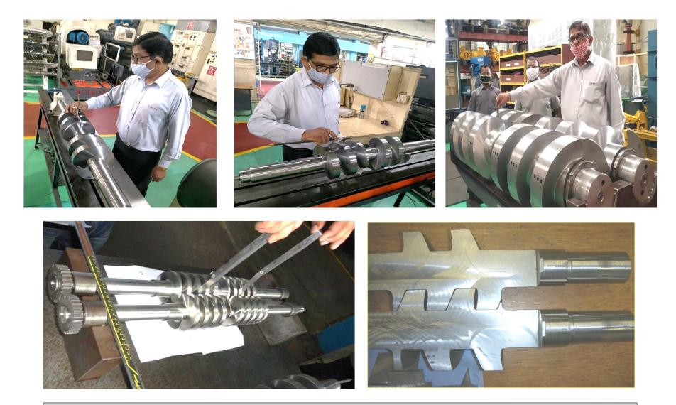
**Checking of Critical to Quality Dimensions and Clearances of Rotors**
