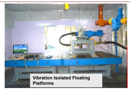
Facility to check 'Air Borne Noise' and 'Structure Borne Noise' as per MIL standards
